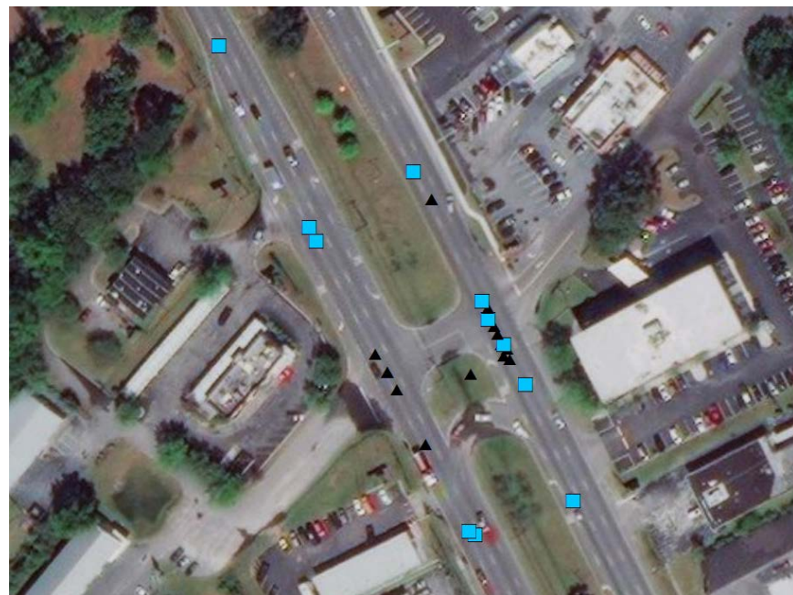
Example of Sideswipe (blue) and Angle (black) Crashes at Rivers Avenue at Hawthorne Drive Crossover
