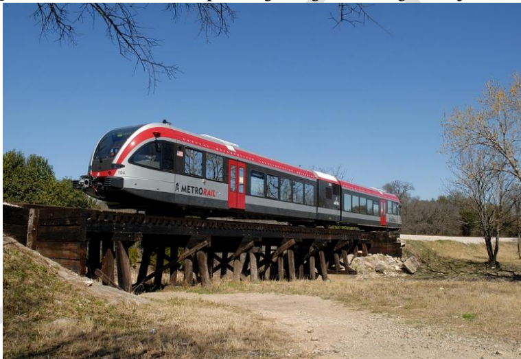
Figure 5 - 3: MetroRail DMU railcar operating along a rural segment of the rail alignment
