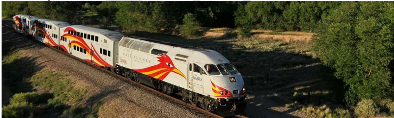
Figure 4 - 2: NM Rail Runner Diesel Electric Locomotive with Bombardier Bi-Level Coaches
