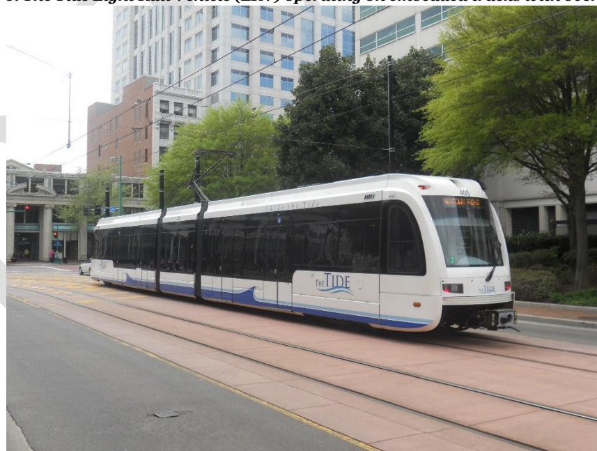
Figure 3 - 6: The Tide Light Rail Vehicle (LRV) operating on embedded tracks with overhead wires
