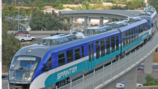
Figure 5 - 4: Sprinter DMU vehicle operating on elevated track
