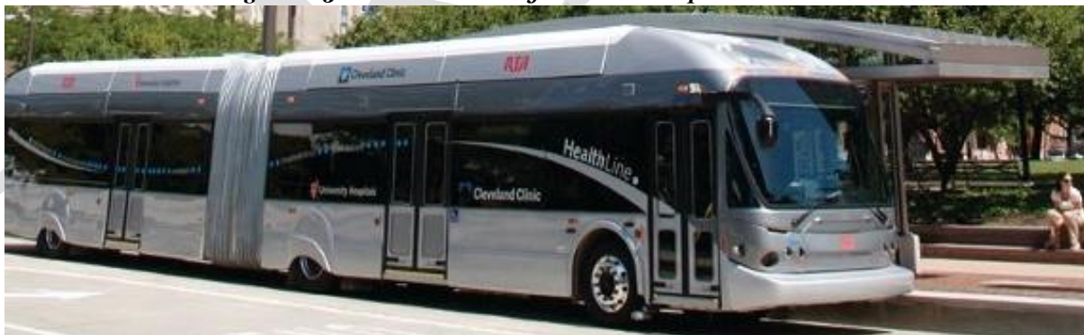
Figure 2 - 3: HealthLine BRT hybrid electric rapid transit vehicle
