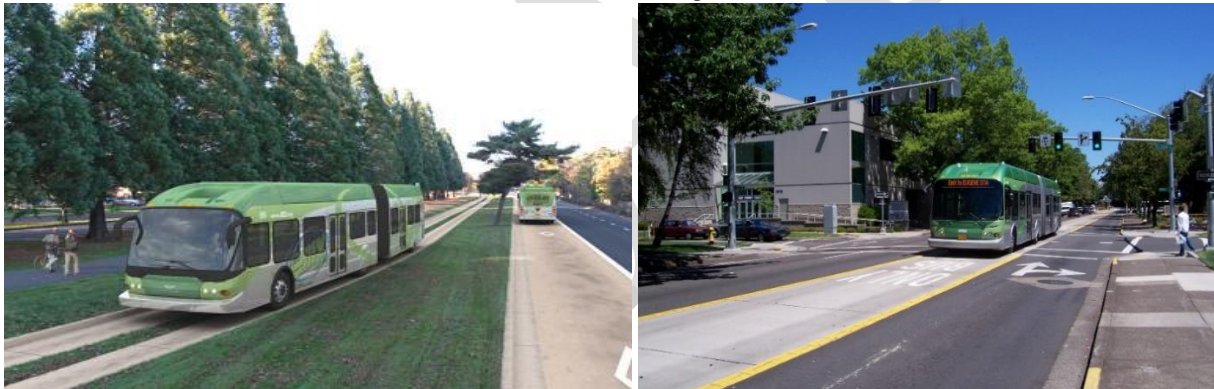
Figure 2 - 11: EmX vehicle operating on dedicated curb-guided bus lanes with grassed median strip (left), and median bi-directional lane (right)
