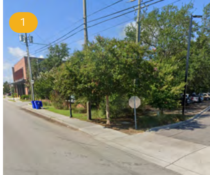
King St Ext has a continuous sidewalk on its western side, but it lacks detectable warning strips, high-visibility crosswalks, and buffers.
