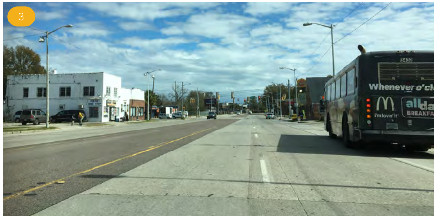
Rivers Ave is a 5-lane road with striped bicycle lanes that are used as curbside on-street parking and bus pullout space. Several bicyclists were observed biking on the sidewalk instead of in the bicycle lanes, indicating that the existing bicycle lanes do not provide a sufficient level of comfort for current users.
